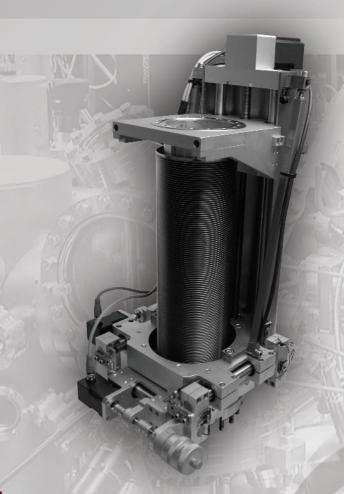
The HPM 100S is a shorter design of Omnivac's HPM 100 standard manipulator.
